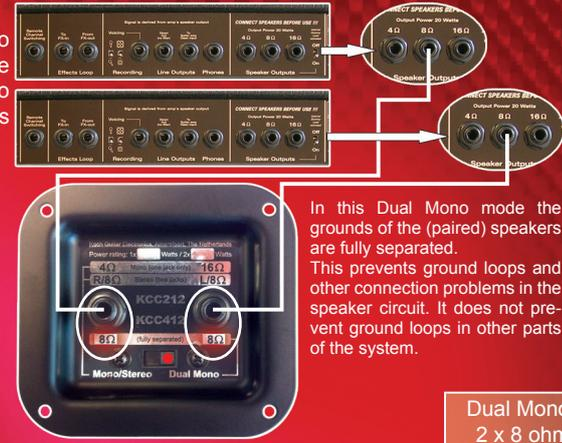
In this Dual Mono mode the grounds of the (paired) speakers are fully separated. This prevents ground loops and other connection problems in the speaker circuit. It does not prevent ground loops in other parts of the system.
