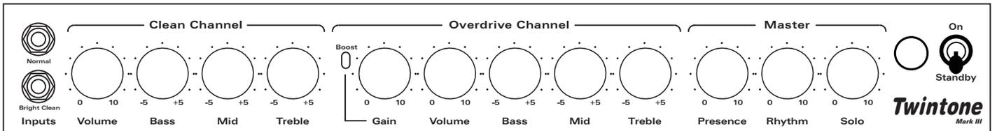
Diagram of the Twintone Mark III control panel. It features two input channels: Clean Channel and Overdrive Channel. The Clean Channel has four knobs for Volume, Bass, Mid, and Treble. The Overdrive Channel has a Boost switch and four knobs for Gain, Volume, Bass, and Treble. The Master section has three knobs for Presence, Rhythm, and Solo. There are also two On/Standby switches. The Twintone Mark III logo is in the bottom right corner.
